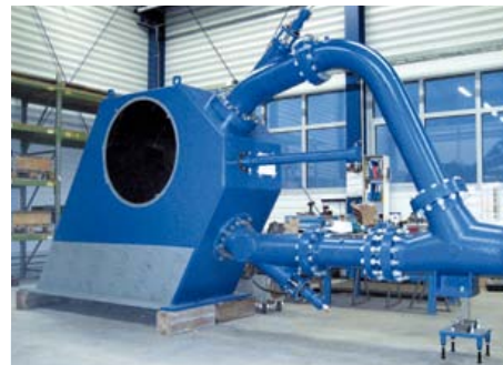
ELANDSRAND HPP, South Africa 1 horizontal 2 nozzle Pelton D_1 = 675 mm P = 3.8 MW, H = 620 m
