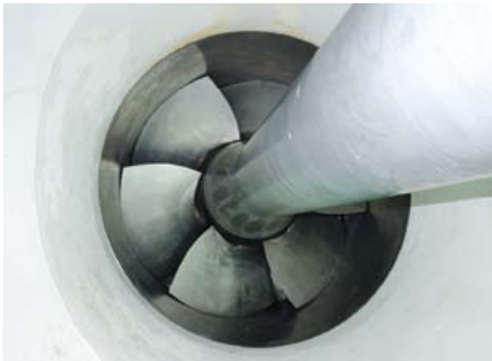
UMBATA HPP, Canada 2 Axial S-Type D_1 = 2,200 mm P = 2 \times 11.7 MW, H = 34.1 m
